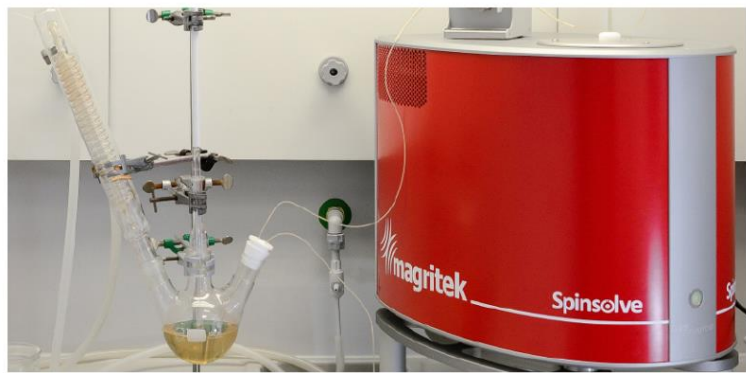
Hydrolysis of acetic anhydride with mass balance (see Magritek Application Note 9)
